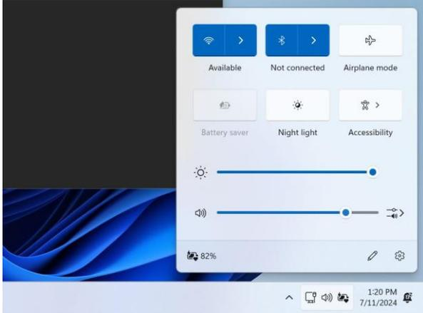
If this is not displayed when the speaker icon is pressed, click on the arrow next to the volume bar to expand the device names and select the Extron HDMI (HD Audio Driver for Display Audio).
