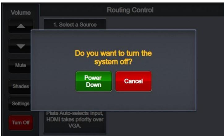
Press **Power Down** and the projector will turn off, and the screen will raise back up into the ceiling.
